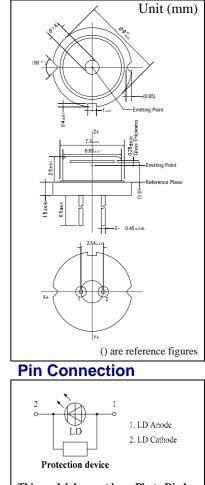
This model does not have Photo Diode. This model has a protection device built in as a protection circuit against static electricity.
